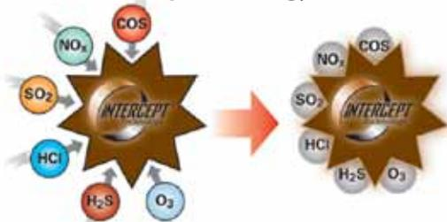
Intercept delivers protection by reacting with and then permanently neutralising the corrosive elements.
